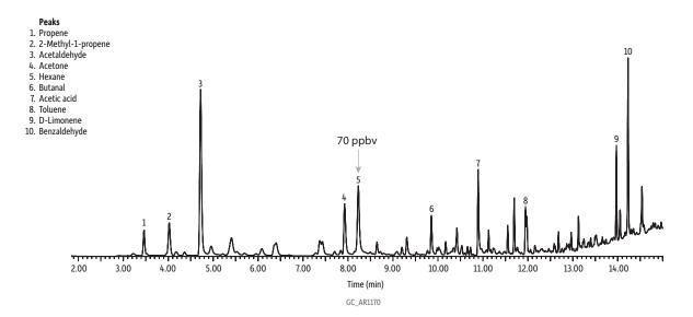
Rtx-VMS, 60 m, 0.25 mm ID, 1.40 µm (cat.# 19916) Column with MXT low-dead-volume connector (cat.# 20536)
