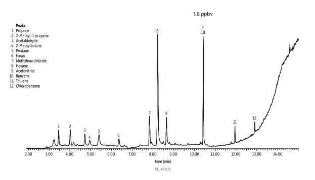
Column Rtx-VMS, 60 m, 0.25 mm ID, 1.40 µm (cat.# 19916) with MXT low-dead-volume connector (cat.# 20536) Shipping facility air sample
