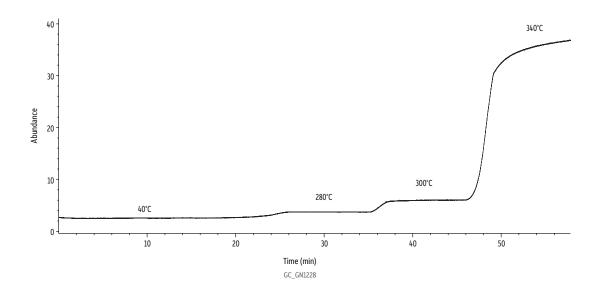
Rtx–200ms, 30 m, 0.25 mm ID, 0.25  $\mu m$  (cat.# 15623) Instrument blank Column Standard/Sample
