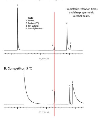
Comparison of competitor column and Rtx-DHA-100 column, 100 m, 0.25 mm ID, 0.50  $\mu m$  (cat.# 10148) Column
